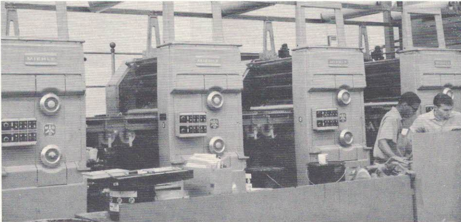
These four printing units represent eight presses! Each unit prints on both sides of the page at once. From left to right, the units print yellow, magenta, blue and black, respectively—the primary colors in the four-color, full-color process.
