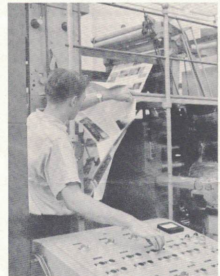
These four printing units represent eight presses! Each unit prints on both sides of the page at once. From left to right, the units print yellow, magenta, blue and black, respectively—the primary colors in the four-color, full-color process.
